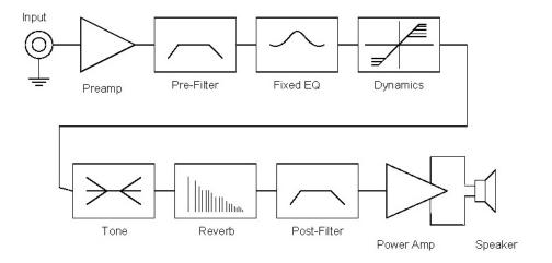
Figure 1: Block Diagram
