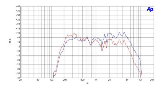
Figure 6: Acoustical Frequency Response and Tone Control Range
